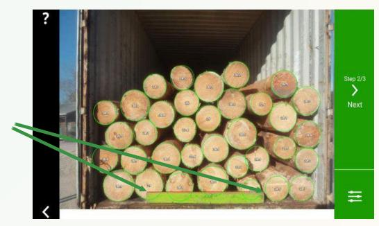
7. As a final step, in case of a missing log or another circular object detected, add/remove circle by holding finger on the screen.
